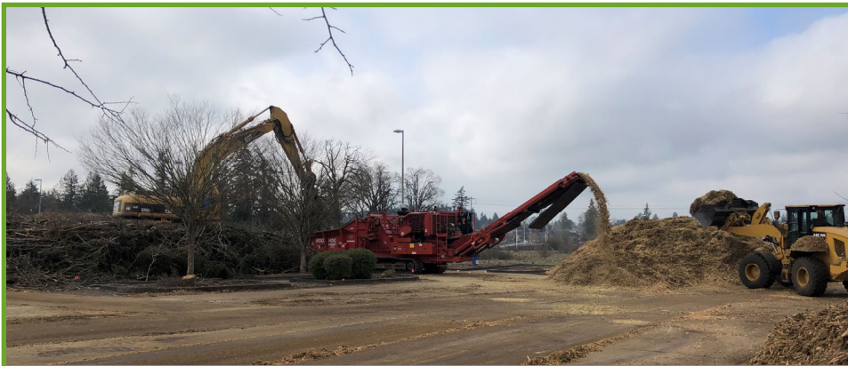
Super-sized tub grinder making wood chips
