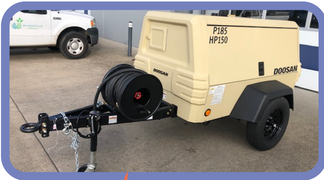
The City's new 150 PSI portable air compressor
