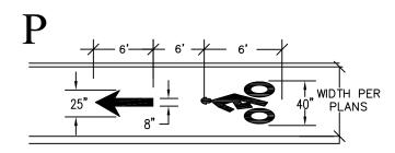
BICYCLE LANE MARKING: SEE ODOT BIKE LANE STANDARDS. USE PREFORMED METHYL METHACRYLATE (MMA) PAVEMENT MARKING MATERIAL.
