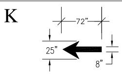
BICYCLE LANE ARROW: SEE ODOT BIKE LANE STANDARDS. USE PREFORMED METHYL METHACRYLATE (MMA) PAVEMENT MARKING MATERIAL.
