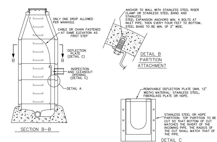
1. MANHOLE TO CONFORM WITH DETAIL S-2005.
