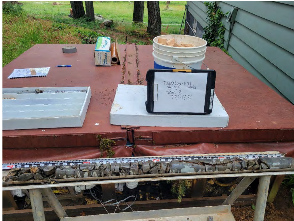
BORING B-3, CORE RUN 2, 7.5 TO 12.5 FEET BGS.
