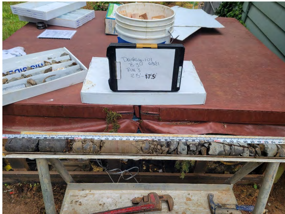
BORING B-3, CORE RUN 3, 12.5 TO 17.5 FEET BGS.
