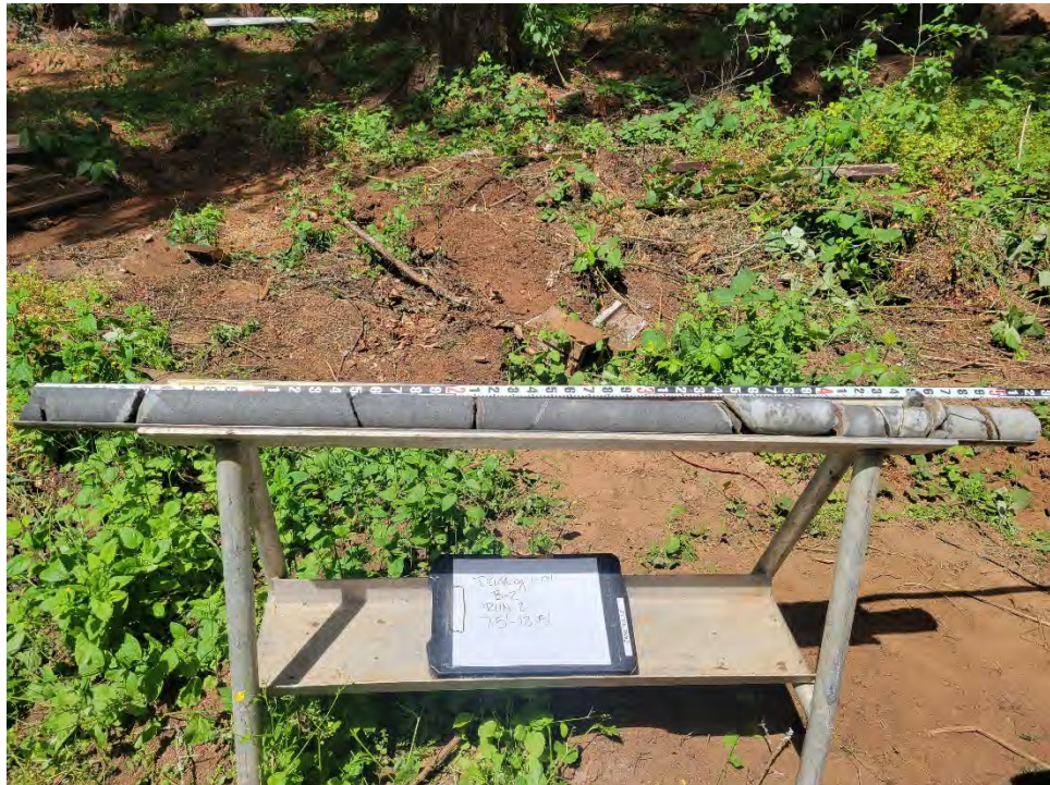
BORING B-2, CORE RUN 2, 7.5 TO 12.5 FEET BGS.
