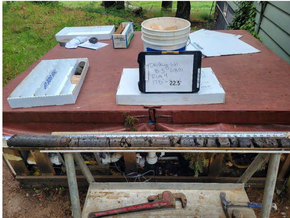
BORING B-3, CORE RUN 4, 17.5 TO 22.5 FEET BGS.
