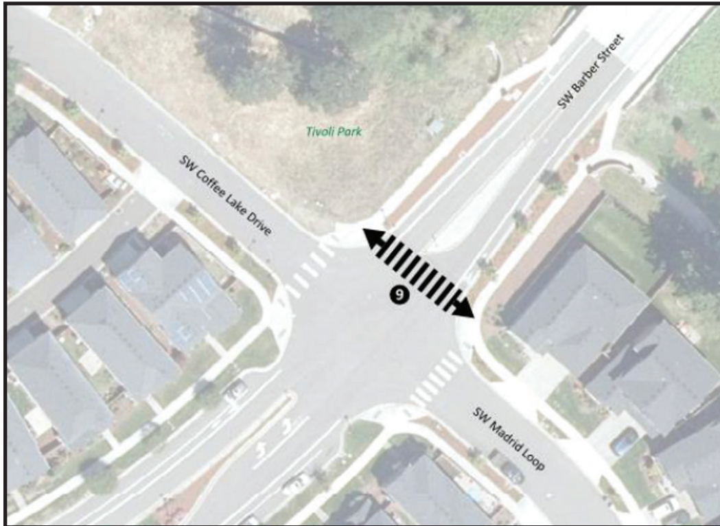
Planned pedestrian crossing enhancement at Barber Street near Coffee Lake Drive (CIP #4717).
