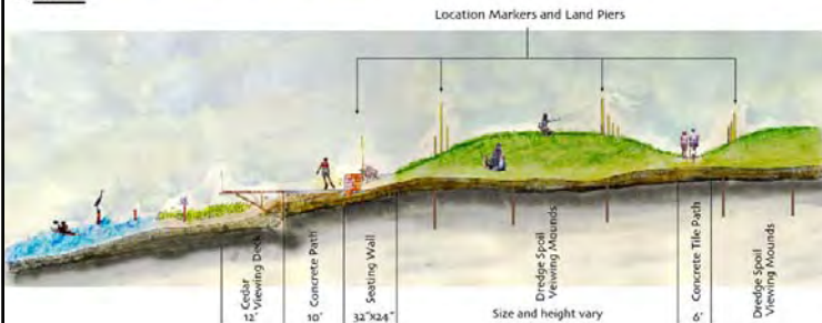
Section Elevation Boardwalk, Viewing Mounds and Location Markers scale 1"=8'
