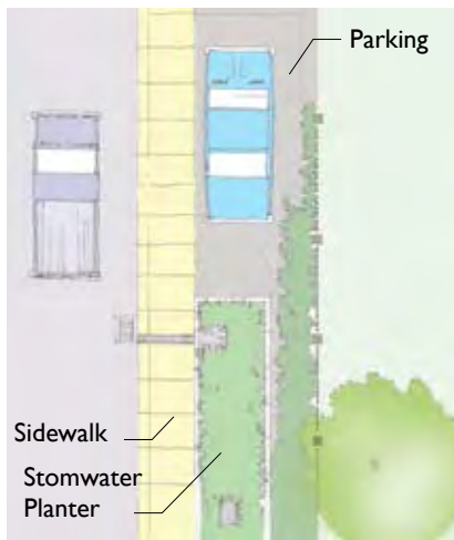
Figure 18: On-Grade Sidewalk and Stormwater Planter
