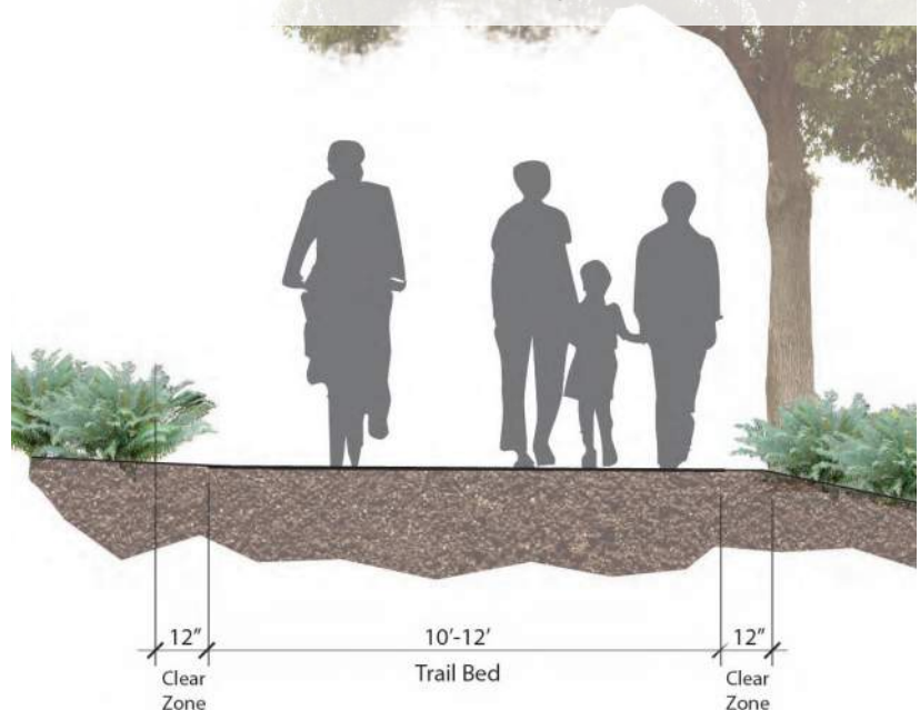
Figure 32. Boeckman Creek Regional Trail Cross-Section
